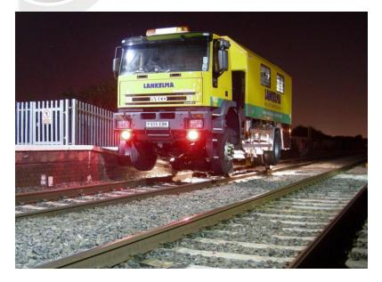
Lankelma was asked to undertake a site investigation on the rail tracks near Bolton in the first quarter of 2014. Using the 19 tonne road-rail vehicle, UK12, Lankelma drove to the set road rail access point, deployed the turntable and bogies to get on track and then began testing within the four-foot.
